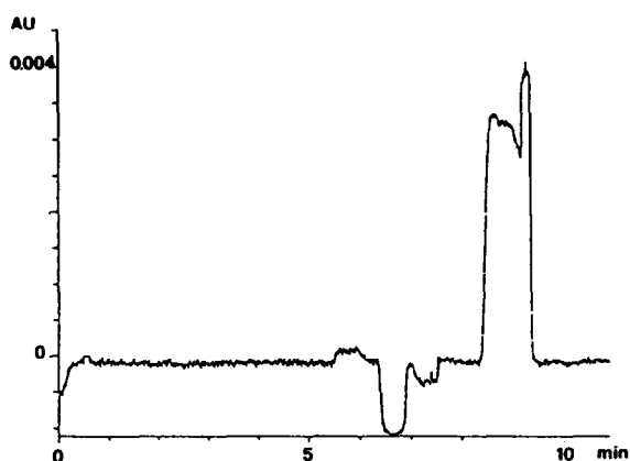
Fig. 6. Electropherogram of the re-injected pooled fraction (nine separations with 40-s pressure injection and a sample concentration of 4 \text{ pmol/nl} ) of 2'dT: 60-s pressure injection, approximate concentration 0.34 \text{ pmol/nl} .
